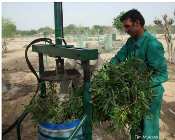
Fig 1. Drum being filled in the browse press.
