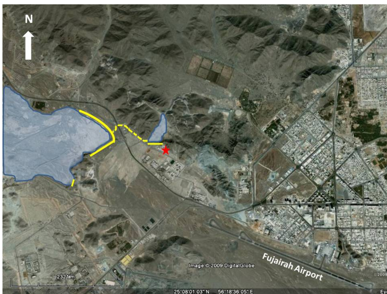
Figure 1. Location of the Ham dam complex in Fujairah. The dam is shown in yellow solid line. The dash yellow line shows the spillway collecting the discharge of the main dam to the auxiliary dam "D" near the Fujairah Tennis and Country Club (indicated with a red star).
