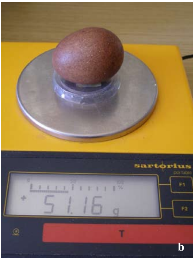
Photos 2a, b, c, d. Equipment used to measure the eggs. Egg length and width was measured with the calliper (a), egg mass with an electronic balance (b), egg hardness with an isometric Kistler force transducer (c) and eggshell thickness with a micrometer (d) (Aurora M. Castilla)
